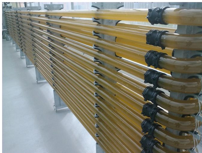
Photobioreactor at A4F Pilot Unit located in Lisbon.
